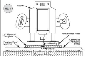
2. Start router about 1 in. (25.4 mm) away from edge of template and pull or cut back to template cut out area so bearing is riding against inside of template. Plunge or gradually cut down to foam pad using several passes around template. Do not cut through foam, cork, or floating floor pad. Carefully remove template by pulling back on the tape tabs, and clean out routed area thoroughly.
