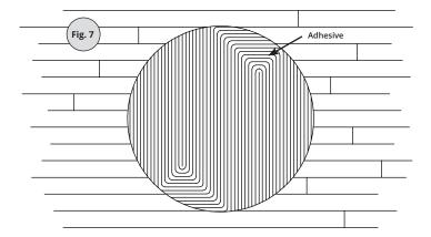
**9.** Place stone medallion (stone side up) onto adhesive and press into place so stone medallion is flush and level with surrounding wood floor. When properly positioned, there will be a  $\frac{3}{16}$  in. (5 mm) gap between the stone and the surrounding wood floor.
