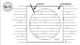
**New Construction: 1b.** Place the stone medallion on the subfloor in the desired location. Draw a pencil line on the subfloor around the stone medallion. Measure from two walls to the pencil line and write down these measurements on the template, so you can place the stone medallion in the same place when the pencil lines are covered up.
