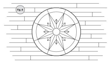
**10.** Allow the adhesive to set for 24 hours. For easier clean up, tape over the expansion joint with masking tape and trim tape with a utility knife so only the joint is exposed. Fill the expansion joint between the stone medallion and the surrounding wood floor with the silicone acrylic latex caulk provided. Remove the tape, and then use a damp cloth to clean caulk from surrounding area, being careful not to touch caulked seam.
