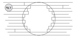
**3.** Position the plywood installation template over the pencil line. If the line is on the subfloor (now covered with flooring), use your measurements from Step 1 to help position the template. Secure the template to the floor, using the adhesive 3M tabs (double-stick tape) provided.
