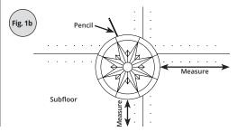
**2.** Begin installation of your hardwood flooring. When you reach the stone medallion outline on the subfloor, overlap the line by 1 to 2 in. (25 to 50 mm) with the flooring, being sure to nail each flooring board about 1 to 2 in. (25 to 50 mm) **outside the line**. To avoid hitting nails with the router bit, do not nail on or inside the pencil line.
