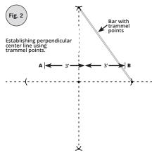
From the points at which the arcs intersect with the Primary working line, adjust the trammel point beam or bar compass to 5 feet and scribe arcs in the general area of where the 90-degree Secondary Line will be. Do this both above and below the Primary working line.
