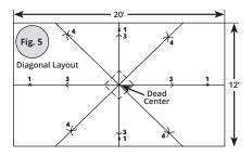
**1.** Mark on the subfloor along the 20 ft. (6096.0 mm) walls at the middle or 10 ft. (3048.0 mm) point of the room. Snap a chalk line between these two points to establish a primary line.
