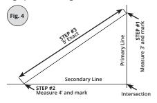
Measure three of anything: feet, yards, or any unit. Use feet-yards (meters) in big rooms. Measure 36 in. (914.4 mm or three units) on one line. Mark 48 in. (1219.2 mm or four units) on the other and measure the distance between marks. It should be 60 in. (1524.0 mm or five units) exactly. If not exactly 60 in. (1524.0 mm or five units), adjust the secondary line by pivoting on the intersection point until the diagonal reads
