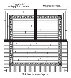
**Note:** To complete the installation up to the wall or your expansion space, you should top nail (or glue) the last frame around the apron. Use base molding to cover nails.
