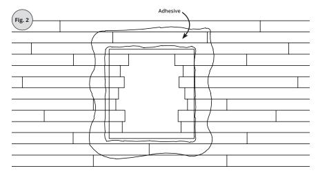
**3.** Fasten the template to the field flooring. The template can be fastened with 3M tabs provided, or by finish nailing into the field flooring between the floor boards.
