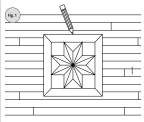
**Note:** Use magnets to find any fasteners along the outline and mark them. A template is provided, thereby reducing the chance of making bad cuts outside the proposed area for the inlay. Pay attention to small pieces of the floor that may be on the edge of the cutout area.
