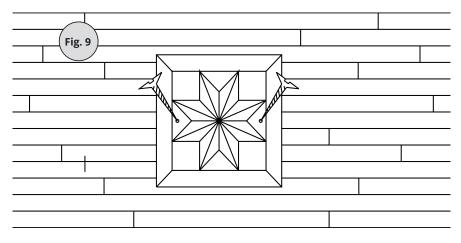
**9.** Glue the knock-out pieces into their original places using woodworker's glue or urethane adhesive. Allow adhesive to dry for 24 hours.
