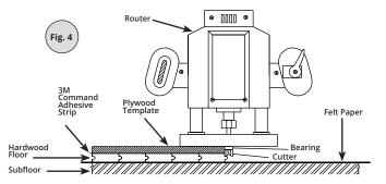
With router running, plunge the bit into the flooring, about an inch inside the template. This will prevent possible damage to the template when you insert or start your cutting into the floor. Pull the bit snugly against the template so the bearing makes contact with the inside wall of the template, then make your first cut in a clockwise direction. Move the router slowly, giving it time to
