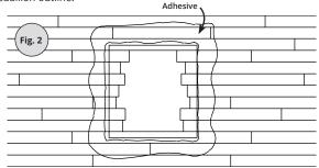
**3.** Fasten the template to the field flooring. The template can be fastened with 3M tabs provided, or by finish nailing into the field flooring between the floor boards.
