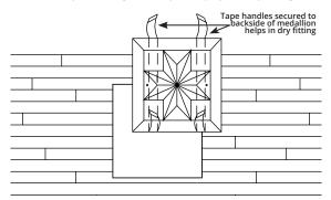
**6.** Using adhesive, bead even lines (½ to ¼ in. diameter) of adhesive approximately every 1-½ to 2 inches onto subfloor into cut-out area. **Use only as much adhesive as necessary to cover cut-out area.**
